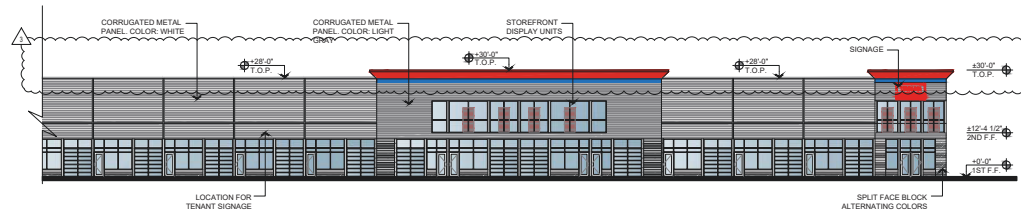
BIG HORN BLVD ELEVATION CONT. ② 1/16"=1'-0"
